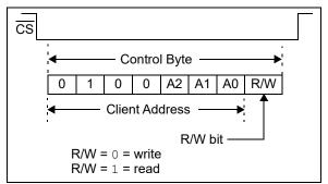
FIGURE 3-5: SPI Control Byte Format.
