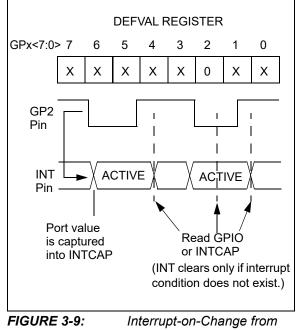
**FIGURE 3-9:** Interrupt-on-Change from Register Default.
