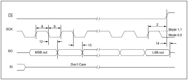
FIGURE 1-6: SPI Output Timing.
