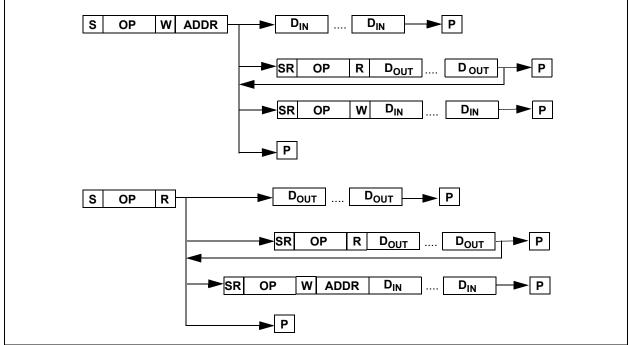
FIGURE 3-3: MCP23017 I<sup>2</sup>C Device Protocol.
