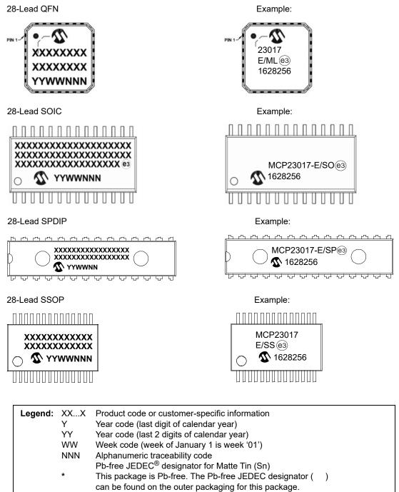
•, ▲, ▼ Pin one index is identified by a dot, delta up, or delta down (triangle mark).
