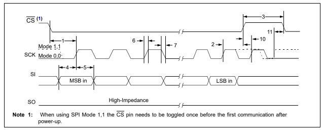
FIGURE 1-5: SPI Input Timing.
