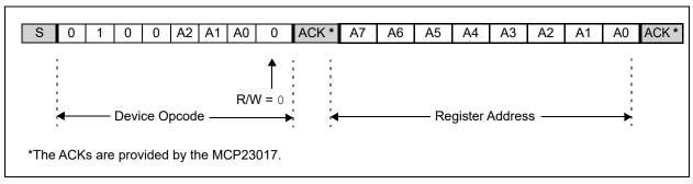
FIGURE 3-6: I<sup>2</sup>C Addressing Registers.
