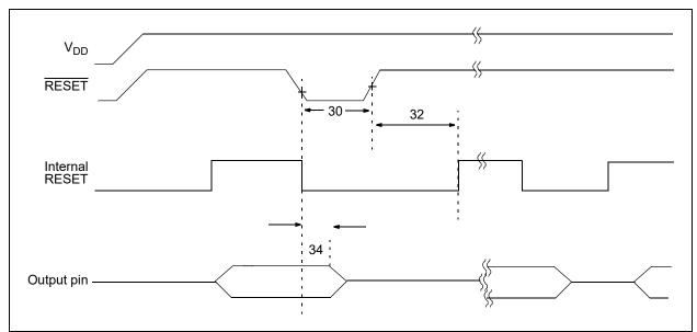
FIGURE 1-2: RESET and Device Reset Timer Timing.
