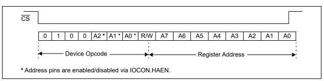
FIGURE 3-7: SPI Addressing Registers.
